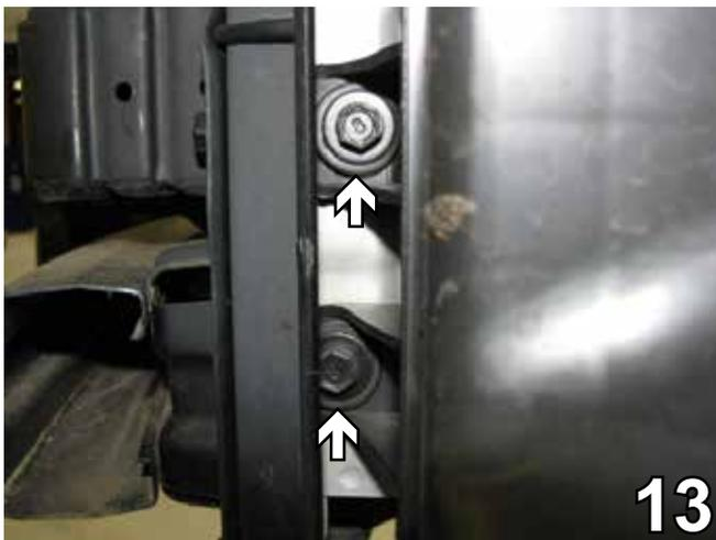
13. On the driver's side, using a 12MM socket remove two bolts from the front side of the air intake baffle. Set bolts aside to be reinstalled later.
