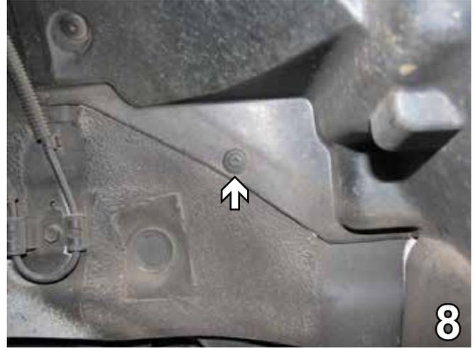
8. On the passenger side only, remove the plastic Phillips push pin, in order to press the wheel well cover toward the tire to expose two metric bolts. Set pin aside to be reinstalled later.
