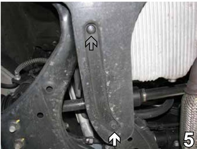
5. On the passenger side, remove another push pin (gray arrow). Using a 12MM socket, remove the bolt (white arrow). Set push pin and bolt aside to be reinstalled later.
