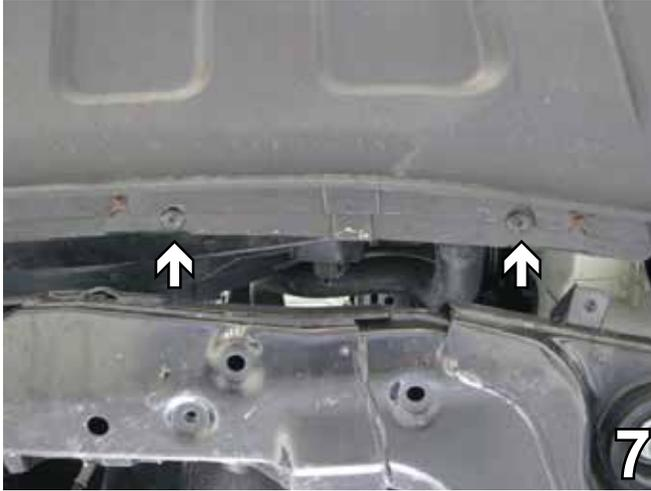
7. Remove four Phillips push pins from the bottom of the fascia. Set fascia and push pins aside carefully to be reinstalled later.
