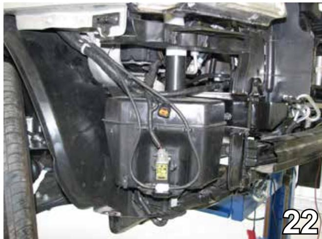
22. Reinstall windshield washer reservoir to its original position. Reconnect electrical and water lines to windshield washer reservoir.
