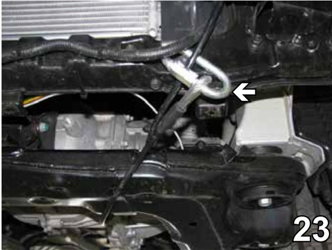
23. Attach the permanent baseplate safety cables to the provided convenience link on the baseplate. The photo above shows the recommended installation of the cables to frame of vehicle. Additional options may interfere with suggested mounting; in this case secure the cables to a solid piece of the frame as described in the instructions included with the permanent baseplate safety cables. Be sure the safety cables do not rub against any hoses or moving parts.
