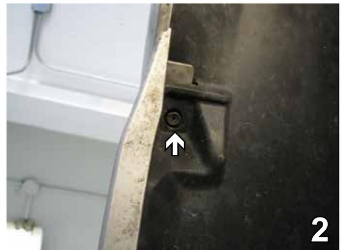
2. Just inside the wheel well, on the edge of the fascia, remove one metric bolt with an 8MM socket. Do this to both sides of the vehicle. Set bolts aside to be reinstalled later.
