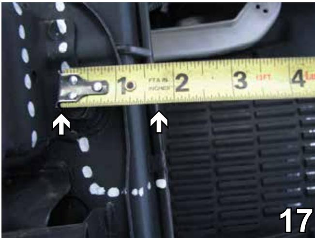
17. The section is flush with the frame rail on the top and 1 3/4" across. Do this on both sides of the vehicle.
