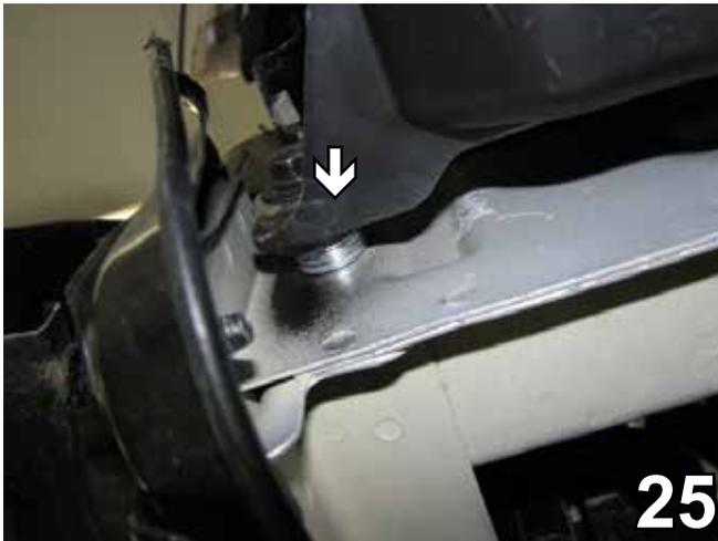
25. Reinstall the air baffle. Add eight 1/4" flat washers for the two bolts to space the baffle out and miss hitting the two previously installed bolts.
