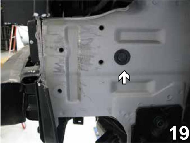
19. Remove the rubber grommet from the frame rail.
