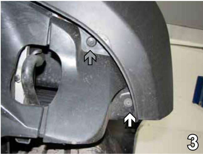
3. Just forward of the front tire on the fascia up underneath in the corner, using an 8MM socket remove one bolt (white arrow). Remove one Phillips push pin (gray arrow). Do this to both sides of the vehicle. Set aside to be reinstalled later.
