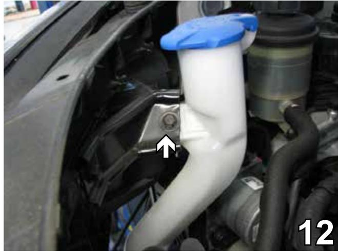
12. Using a 10MM socket, remove one metric bolt from the top spout of the windshield washer reservoir. Guide the windshield washer down and remove from the vehicle set the reservoir and bolt aside to reinstall later.
