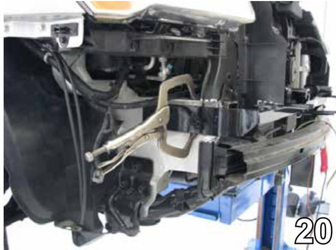
20. Slide the baseplate onto the frame through the opening in the radiator support. Clamp into place using the large vise grips. Using the baseplate as a template, drill three holes in the frame with the 13/32" drill bit. Do this to both sides of the vehicle.
