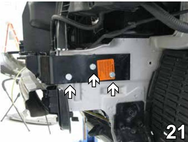
21. Insert three 3/8-16 nut plates through the lower bumper opening and align with drilled holes in the baseplate end plates. Insert the three 3/8-16 x 1 1/2" hex bolts and 3/8" lock washers and fasten to the nut plates. Tighten all bolts with Loctite Red. Do this to both sides of the vehicle.
