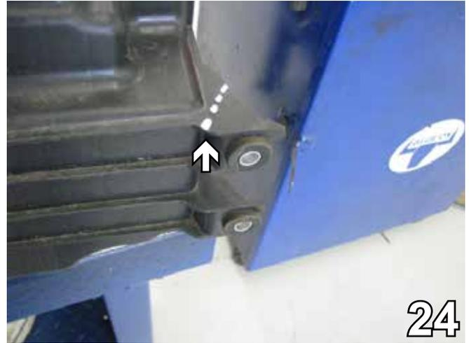
24. Cut the top bracket off of the air baffle.
