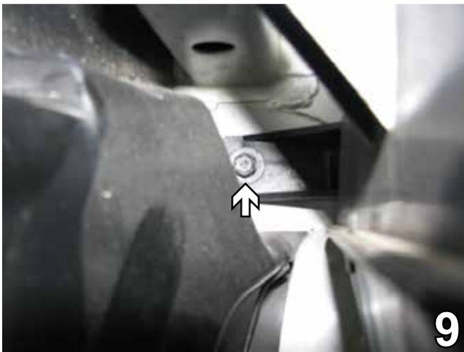
9. Using a 10MM socket, remove one metric bolt from behind the wheel well cover. Set bolt aside to be reinstalled later.
