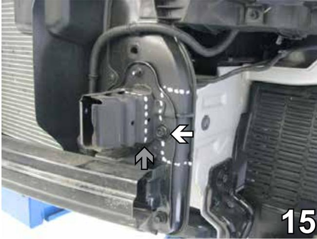
15. Using the 12MM socket, remove one metric bolt from frame (white arrow). Using the reciprocating saw, trim away frame horn end (gray arrow) by cutting vertically just forward of the bracket's rear bolt hole and horizontally along the entire width of the frame horn end and repeating to complete the rectangle. Do this to both sides of the vehicle. Set bolt aside to be reinstalled later.
