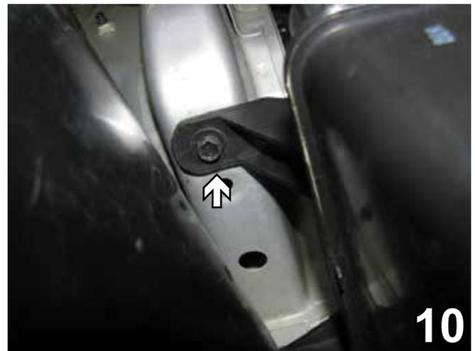
10. Using a 10MM socket, remove another bolt from behind the wheel well cover on the top bracket of the washer reservoir. Set aside to reinstall later.
