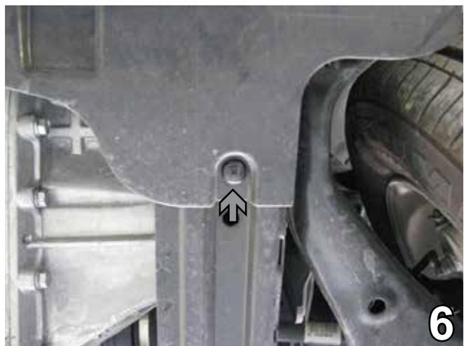
6. On the driver's side, remove only the push pin from the bottom of the fascia. Set belly pan and push pin aside to be reinstalled later.
