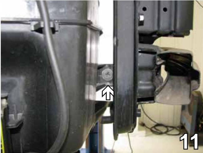
11. Loosen the Phillips screw on the front side of the washer reservoir. Unplug electrical connections, disconnect and plug water lines.
