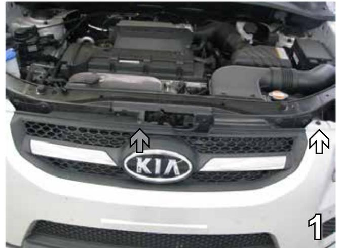
1. Using the 10MM socket remove two metric bolts from top corners of the fascia, see the white arrow in the photo above. Remove one Phillips screw from the top of the fascia, see grey arrow in the photo above. Set all aside to be reinstalled later.
